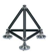
one set-up, probing deviations as well as measuring scale and perpendicularity conditions can be checked. Furthermore, it allows direct comparison of different measuring systems.
