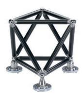
In comparison with the Tetronom, the validity of this artefact in respect of the Z-component is increased because rather than only one ball being measured three balls separated in space are now measured.
